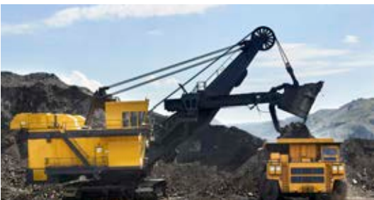
Electric powered mining shovels with TMC transformers on board operating in remote and rugged locations.
