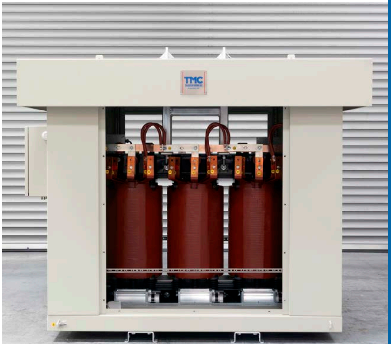
400/480kVA 660/400V LV/LV Cu ANAF IP53 (panels removed)
