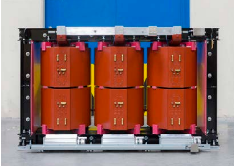
1500kVA 24940-12470/600-208V YNyn0yn0 ANAF 60Hz with 5 limb core
